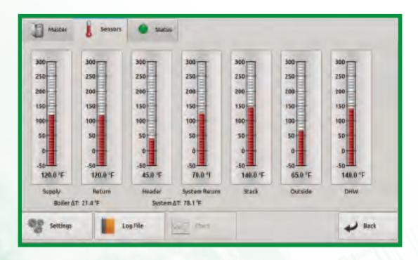
Every KN-Series boiler is integrated with Heatnet 3.0 - an innovative, digital Boiler Management System that provides consistency and feedback through digital communication. By continuously monitoring several system characteristics, HeatNet 3.0 modulates boilier-firing rates to maximize turndown ratios and maintain peak efficiency - no matter the load.
